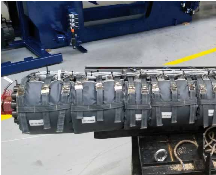
Jacking for heating screws (before final assembly)
