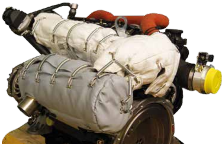
Small ship diesel engine with insulation for different temperature ranges
